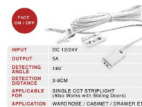
SINGLE DOOR AND SLIDING DOOR IR SENSOR TYPE 3 WITH ADDED FADE ON OFF FEATURE FOR SINGLE CCT LED STRIPS FOR CABINET AND WARDROBE LIGHTING MEM249
